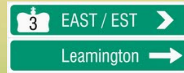
EXIT ROAD ID AND EXIT DESTINATION
